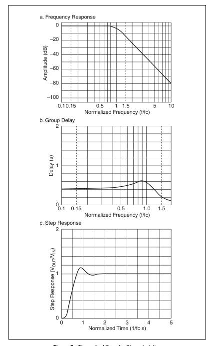
Figure 6. Theoretical Transfer Characteristics
